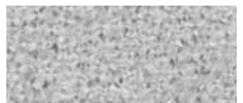
Acrylic Coated Galvalume® (41) 1 SR = 0.67 TE = 0.14 SRI = 56
