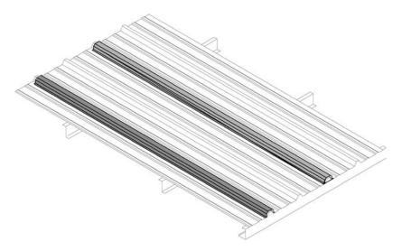
Step 2: Place new Huggers into position ensuring all new sub-framing is square and tightly fitted. Secure the positioning of the Huggers and sub-rafters by installing one 4"-14 at juncture of the two members (Hugger top flange into top of sub-rafter). Begin final attachment of members at juncture of the Hugger and sub-rafter's base flanges for locations that are directly over an existing purlin using 1/2"-14 TEK-3 fasteners at each side of sub-rafter.
