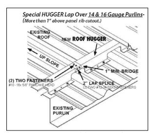
fasteners will replace (2) pancake fasteners provided the clip fasteners penetrate both overlapping flanges of the HUGGER. Higher profile HUGGERS (1" or more of material above the rib cutout) receive (2) #10-16 x 1" (or equal)
