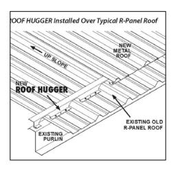
Installing on Existing Corrugated Panels: ROOF HUGGERS Corru-Fit product for existing 2.50", 2.67" and 2.75" corrugated panels up to 1.25" tall is a 2-part system. A 1.25" triangular shaped and a 1.5" spacer tall slotted Spacer/fastener spacing is per engineering design, (2.75" total assembly height). Call ROOF HUGGER for estimated loads and spacing (subject to review). Lap ends are designed to
