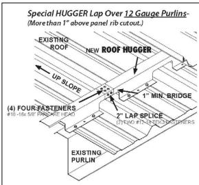
**Grid Framing:** When needed in the corners and edges, hat channel grid framing may be used. Hats that run parallel to the existing panel ribs between the existing purlins are called "Sub-Rafters". They are normally installed 12"- 24" o.c. with (4)  $\frac{1}{4}$ " x 14 x 1 $\frac{1}{4}$ " T3 fasteners into the existing purlins and are designed to transfer the panel loads back to the existing purlins. The hats that run across these members are called
