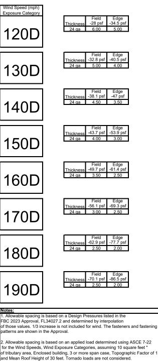
3. Allowable spacing is determined for wind pressure and suction using the combination 0.6W for each.
