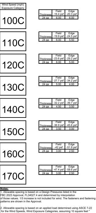
3. Allowable spacing is determined for wind pressure and suction using the combination 0.6W for each.
