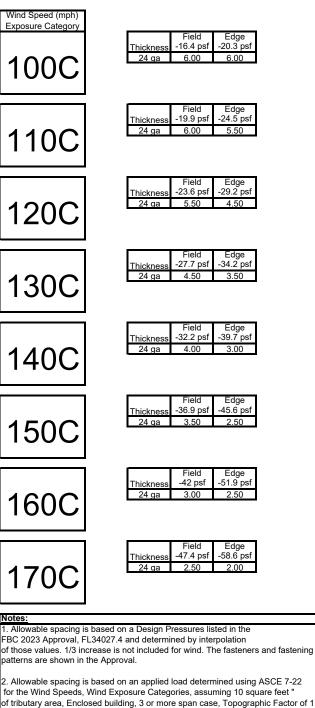
and Mean Roof Height of 30 feet. Tornado loads are not considered. 3. Allowable spacing is determined for wind pressure and suction using the combination 0.6W for each.
