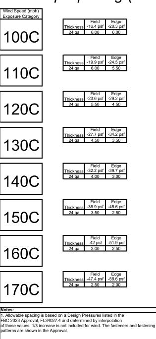
2. Allowable spacing is based on an applied load determined using ASCE 7-22 for the Wind Speeds, Wind Exposure Categories, assuming 10 square feet " of tributary area, Enclosed building, 3 or more span case, Topographic Factor of 1 and Mean Roof Height of 30 feet. Tornado loads are not considered.
