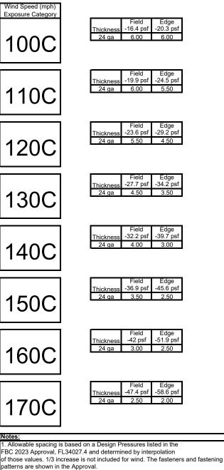
2. Allowable spacing is based on an applied load determined using ASCE 7-22 for the Wind Speeds, Wind Exposure Categories, assuming 10 square feet " of tributary area, Enclosed building, 3 or more span case, Topographic Factor of 1 and Mean Roof Height of 30 feet. Tornado loads are not considered.
