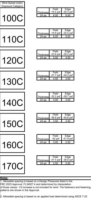
3. Allowable spacing is determined for wind pressure and suction using the combination 0.6W for each.
